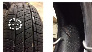
Driving on the tire a short distance while it was severely under inflated caused this dangerous, non-repairable condition shown above. The damage was not visible from the outside. Every tire must be removed from the wheel for inspection and to assess reparability.<sup>1,2</sup>
