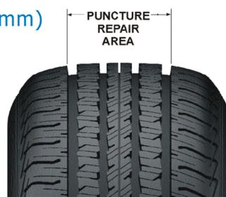
This graphic indicates that puncture repairs are limited to the tread area as generally depicted in the graphic. DO NOT make repairs where the injury damage extends into the shoulder/belt edge area OR where the injury extends at an angle into the shoulder area. If there is any question that the injury extends into the shoulder/belt edge area, then the tire must be scrapped.
