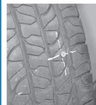
Prior to demounting,<sup>1</sup> check the tire, wheel and valve for the source of the leak(s) by using water or a soap solution. Mark the injured area and totally deflate the tire. Then remove the tire from the wheel being careful to avoid further damage to the tire, particularly to the bead area. Place on a well-lighted spreader. (Avoid excessive spreading of the tire or tire beads.)
