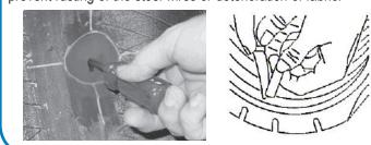
To prevent contamination and preserve the outline, buff within the marked area thoroughly and evenly with a low speed buffer (5,000 rpm max.) with a fine wire brush or gritted rasp. Take care not to expose or damage tire casing body ply cords. Buff to a surface texture per repair material manufacturer's ecommendations.
