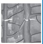
**WARNING** A patch only or a plug (stem) only is an improper repair. Improperly repaired tires can fail while in service. such as by tread-belt separation and/or detachment, which may result in an accident causing serious personal injury or death.
