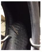
Driving on the tire a short distance while it was severely under inflated caused this dangerous, non-repairable condition shown above. The damage was not visible from the outside. Every tire must be removed from the wheel for inspection and to assess repairability.<sup>1,2</sup>
